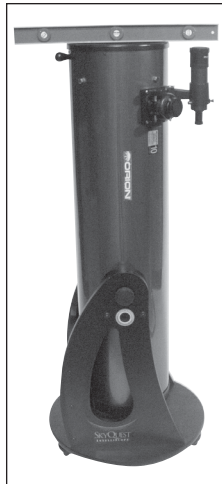
Figure 9. Once the base is leveled, point the tube up until the mirror cell comes into contact with the vertical stop. Then, place the carpenter's level across the top of the tube as shown. If the vertical stop is set properly, the top of the tube should also be level.
