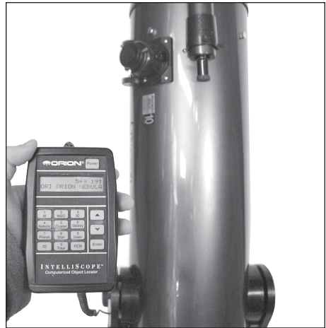
Figure 10. If you stand to the left of the telescope, and face the direction the tube is pointing, the guide arrows will correspond exactly with the direction you should move the telescope in order to find the selected object.
