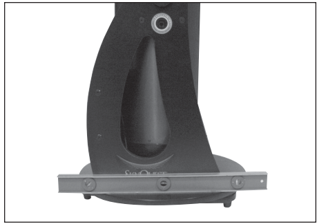
Figure 8. Place a carpenter's level on the base as shown. The base should stay level through a 180° rotation in azimuth. Once the vertical stop is set, the base does not need to be level to function properly.
