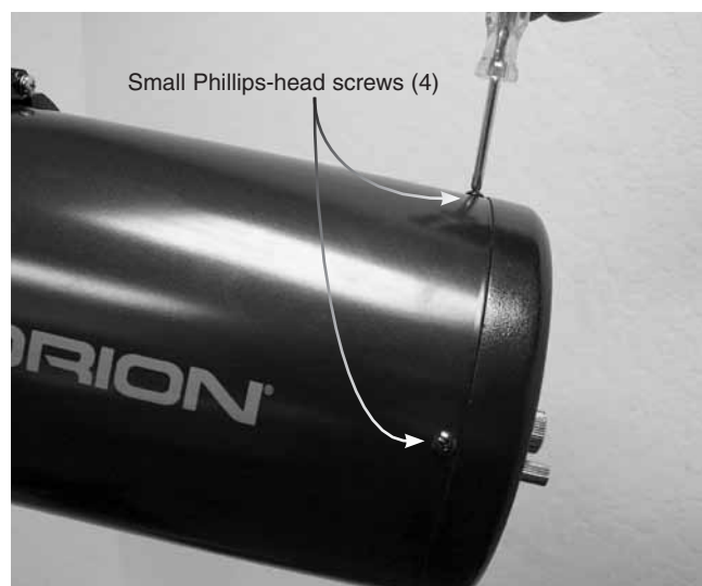
Figure 9. To remove the mirror cell from the telescope, the four small Phillips-head screws on the perimeter of the mirror cell must be completely unthreaded.
