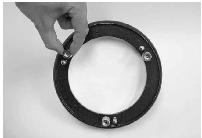
Figure 7. The tilt of the primary mirror is adjusted by turning the three larger thumbscrews.
