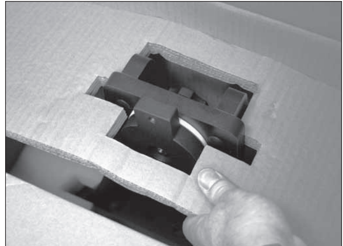
Figure 2. To remove the cardboard insert from atop the altazimuth base, rotate the telescope mounting bracket so its long axis is vertically oriented, then lift the insert off.
