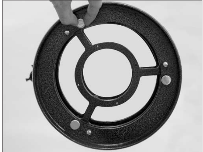
Figure 30. The tilt of the primary mirror is adjusted by turning one or more of the three larger thumbscrews.
