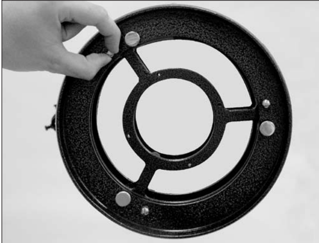
Figure 29. The three small thumbscrews that lock the primary mirror in place must first be loosened before any adjustments can be made.
