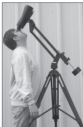
Figure 6. The binocular mount can be used to view objects at or near the zenith. Adjust the tripod so that you can stand under the binocular to view objects located high in the sky.
