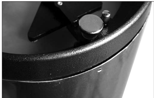
Figure 16. Locate the area of tube that is bulging out and preventing the end ring from fully seating. Press on this bulge to allow the mirror cell to seat properly on the tube. Be careful not to pinch fingers!
