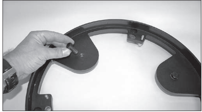
Figure 14. Thread the three hex-head counterweight mounting bolts (XX14g only) into the holes in counterweight support plates as shown. Tighten using an adjustable or 16mm crescent wrench.
