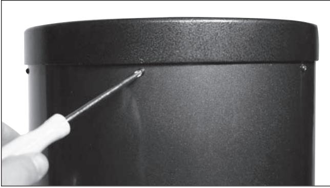
Figure 13. To remove the rear end ring, unthread the Phillips screws that attach it to the tube.
