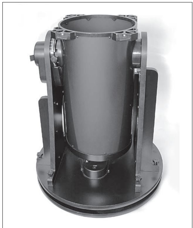
Figure 24. bottom tube section resting vertically in base
