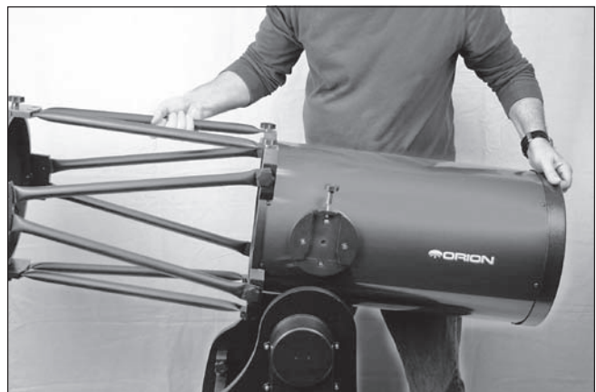
Figure 26. To mount the fully assembled tube assembly onto the base, grasp the rear of the scope with one hand and one of the truss poles with the other. Holding the telescope in a horizontal orientation, lower it into the base, sliding the dovetail slot in the tube’s left altitude bearing onto the mating part of the metal trunion on the left side panel.
