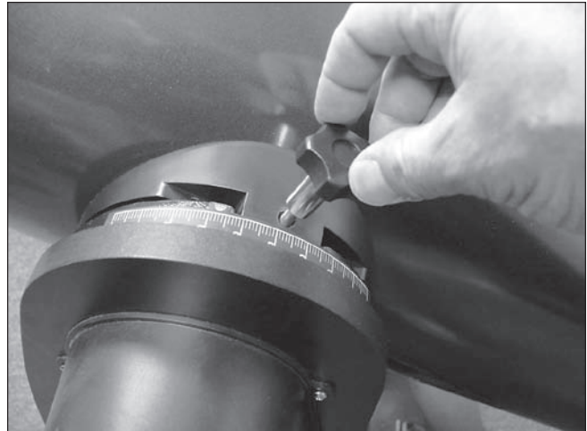
Figure 25. Secure the tube to the base with the tube connecting knob.
