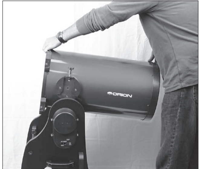
Figure 23. Grasp both ends of the lower tube section to lift it, then lower it into the base, sliding the dovetail slot in the tube's left altitude hub onto the mating part of the metal trunnion on the base's left side panel.
