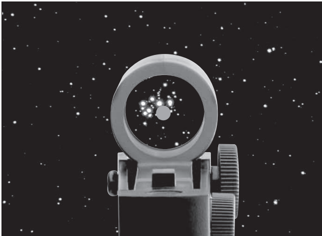
Figure 4. The EZ Finder II superimposes a tiny red dot on the sky, showing right where the telescope is aimed.
