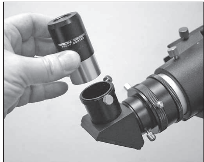
Figure 7. Insert the chrome barrel of the eyepiece into the diagonal and secure with the two thumbscrews.
