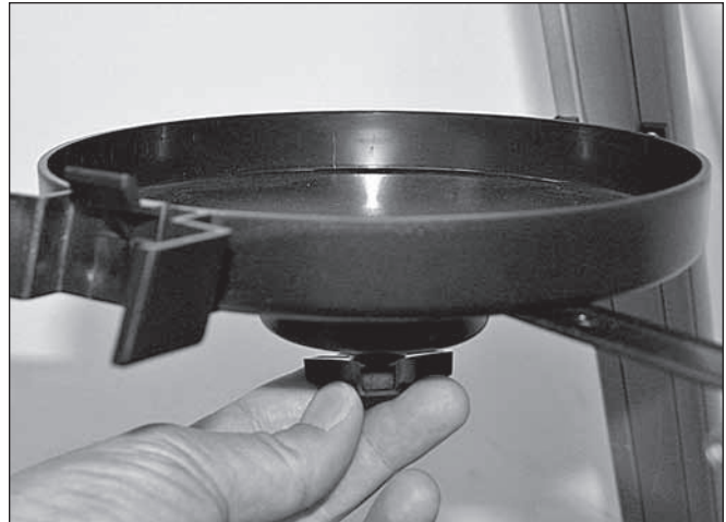
Figure 3. The round accessory tray attaches to the tripod leg brace with the captive screw on the brace.
