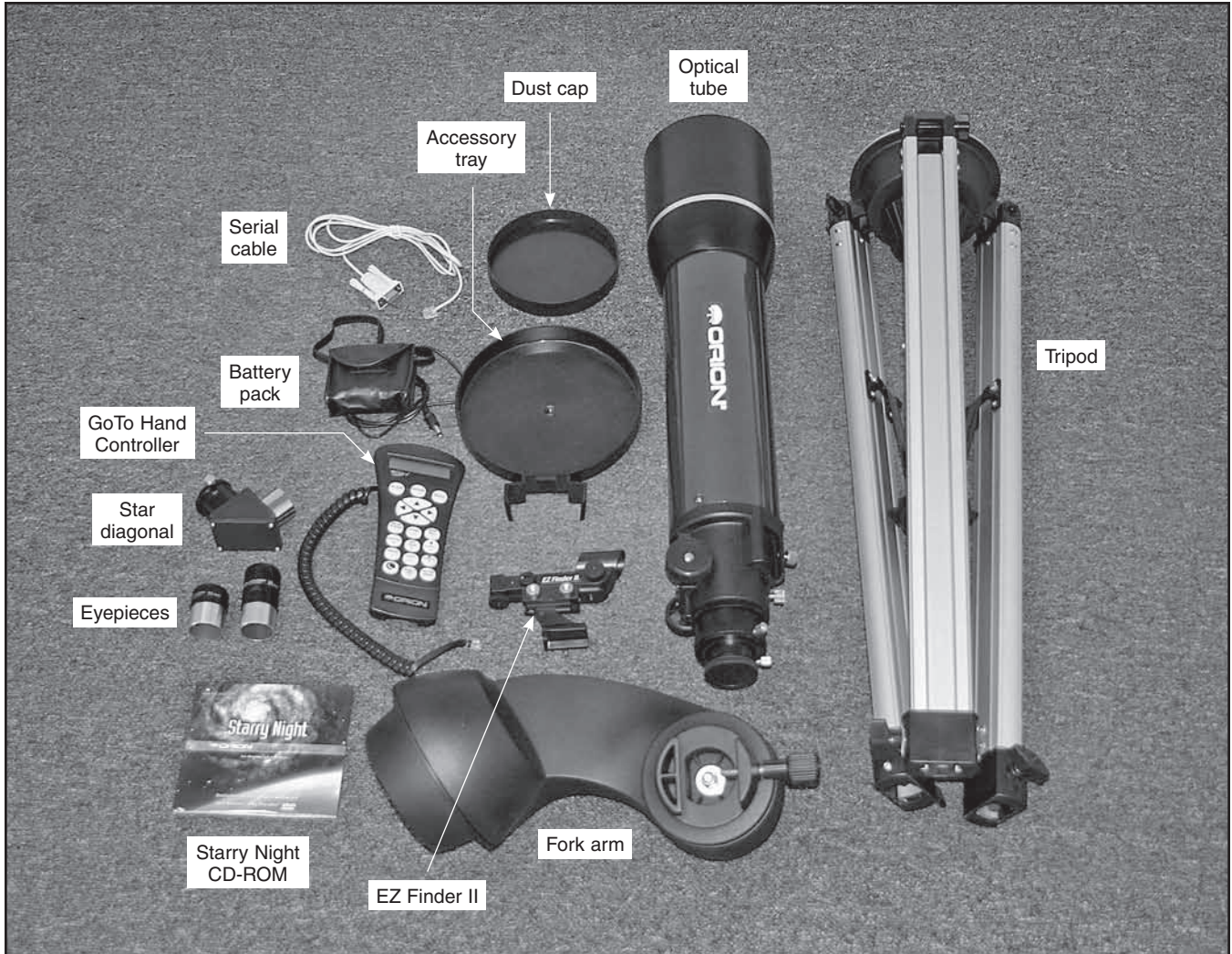
Figure 2. In the box: Parts of the StarSeeker II 102
