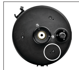
Figure 5. If the view inside the tube shows the black crescent at the bottom, as in Figure 3a , then the first adjustment should be to the pair of collimation screws closest to that direction, as indicated here.
