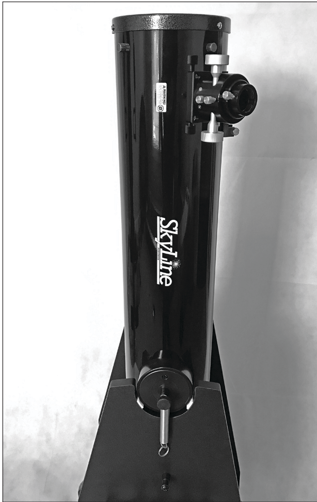
Figure 16. Lift the optical tube and place it in the base as shown.
