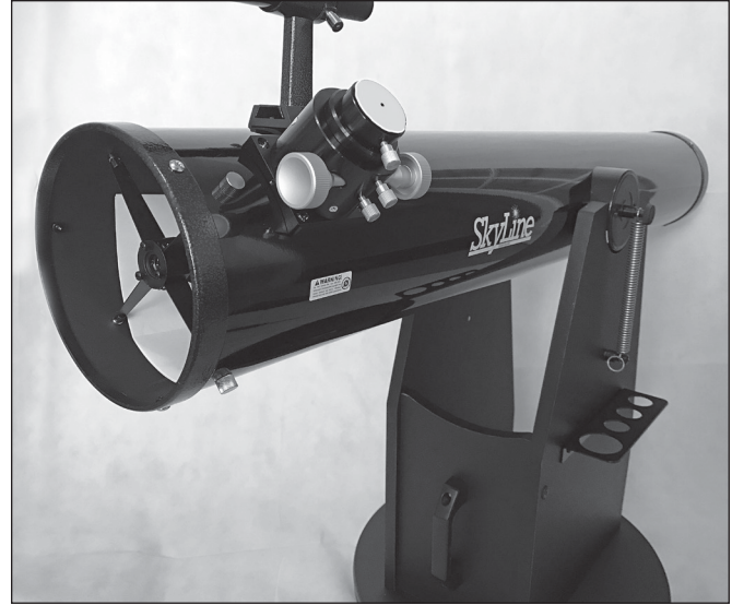
Figure 23. The SkyLine 6" Dobsonian ready for collimation. Orient the tube horizontally and place a piece of white paper inside the tube opposite the focuser.
