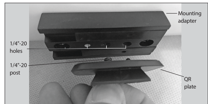
Figure 5. Attach the quick-release (QR) plate to the mounting adapter on the bottom of the telescope optical tube.
