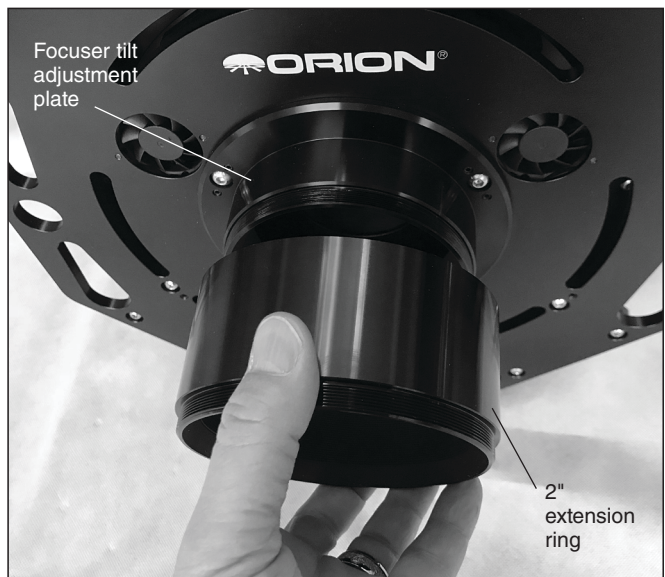
Figure 4. Remove the focuser to thread one or more extension rings onto the focuser tilt adjustment plate, then attach the focuser to the extension ring.
