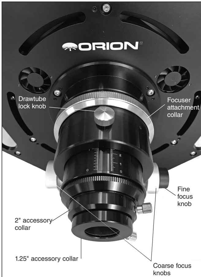
Figure 1. The 3" dual-speed linear bearing Crayford focuser features both 2" and 1.25" compression ring accessory collars.
