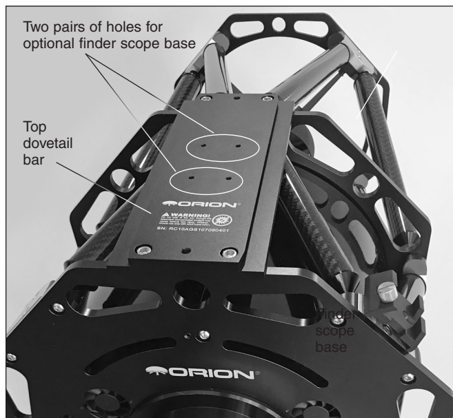
Figure 5. D-style dovetail bars are installed on both the top and bottom of the telescope (top bar shown). Two sets of threaded holes on the bar accommodate an optional Orion dovetail finder scope base.
