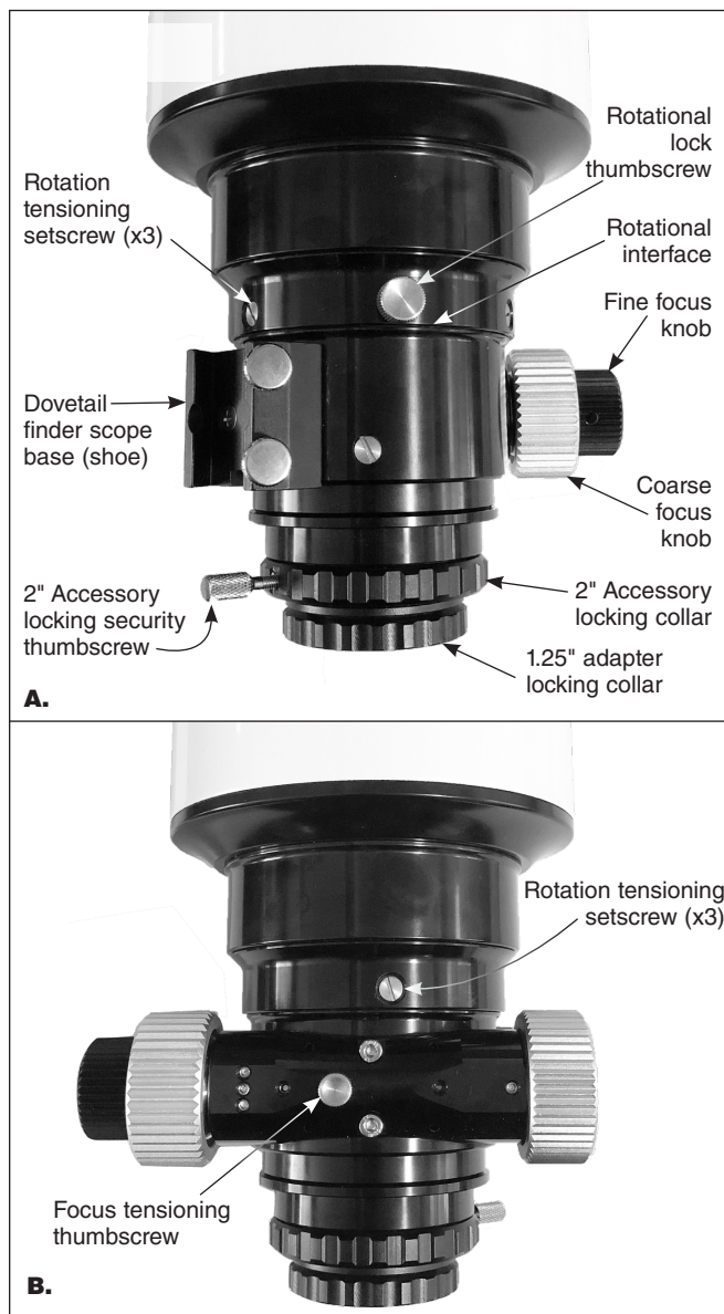
Figure 2. The 2.5" Rack and Pinion focuser used on both the EON 115 and 130 A) Top side, B) bottom side
