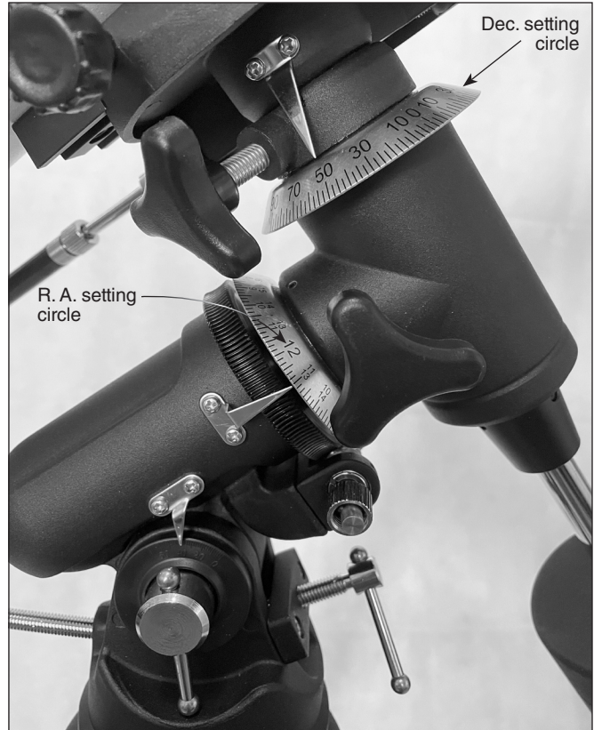
Figure 11. The R.A. and Dec. setting circles allow you to locate an object by its R.A. and Dec. coordinates.
