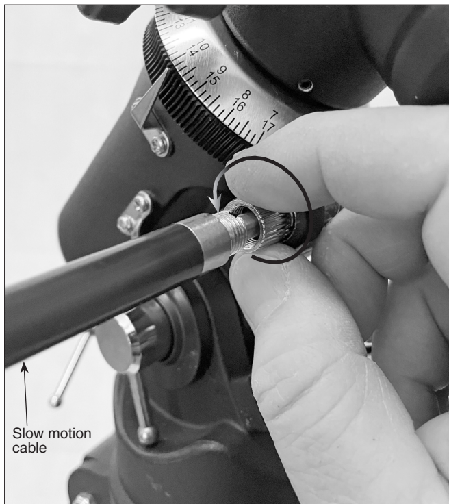
Figure 5. Attach the two slow-motion cables to the mount.
