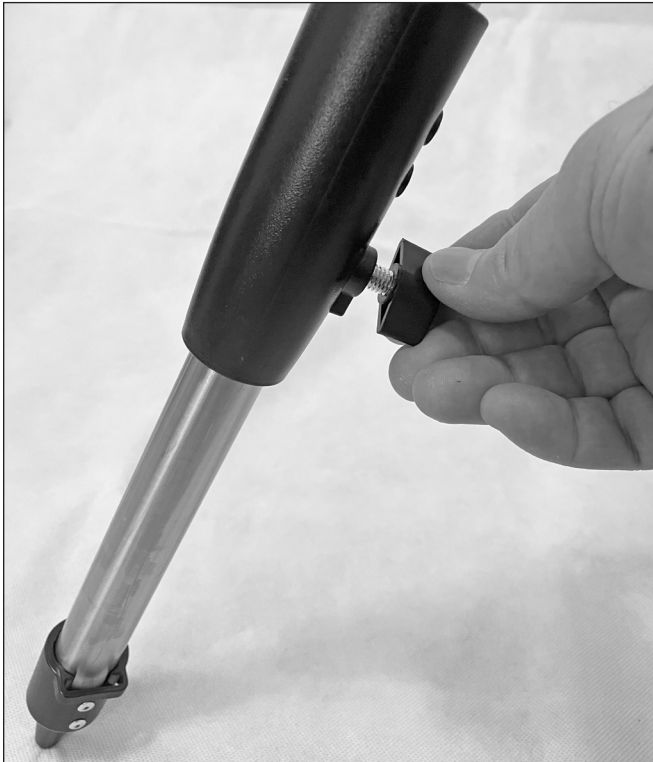
Figure 9. Adjust the tripod leg length by loosening the leg lock knob, then extending the leg to the desired length. Then retighten the knob.
