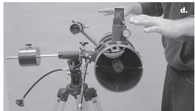
Figure 9. Proper operation of the equatorial mount requires that the telescope tube be balanced on both the R.A. and Dec. axes. (a) With the R.A. lock knob released, slide the counterweight along the counterweight shaft until it just counterbalances the tube. (b) When you let go with both hands, the tube should not drift up or down. (c) With the Dec. lock knob released, loosen the tube ring lock clamps a few turns and slide the telescope forward or back in the tube rings. (d) When the tube is balanced about the Dec. axis, it will not move when you let go.
