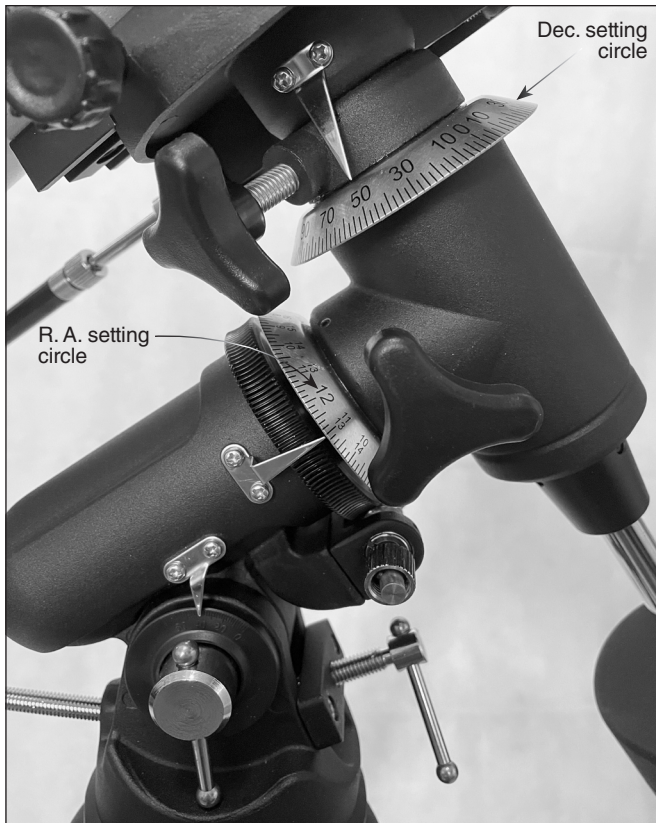
Figure 14. The R.A. and Dec. setting circles allow you to locate an object by its R.A. and Dec. coordinates.
