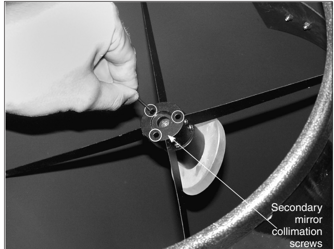
Figure 18. Secondary mirror collimation is performed using the three Phillips screws circled here on the secondary mirror holder.
