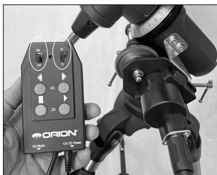
Figure 10. The hand controller features a power switch, and N/S Hemisphere switch, and four speed buttons – forward and reverse - for centering objects in your telescope's field of view.
