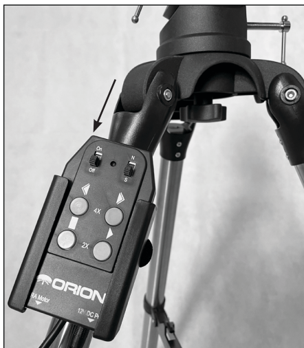
Figure 8. Strap the hand controller holder to a tripod leg with the hook-and-loop band on the back. Slide the hand controller into the top of the holder.
