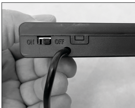
Figure 9. To use the tracking drive you must slide the power switch on the battery holder (and on the hand controller itself) to ON.
