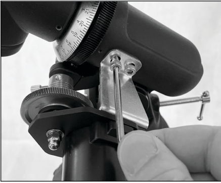
Figure 4. Use the 4mm Allen key to tighten the two socket head cap screws that attach the motor bracket to the mount.
