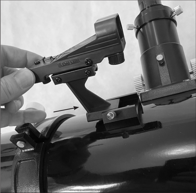
Figure 2. Slide the foot of the red dot scope into the dovetail shoe on the telescope tube, as shown. Then tighten the thumbscrew.
