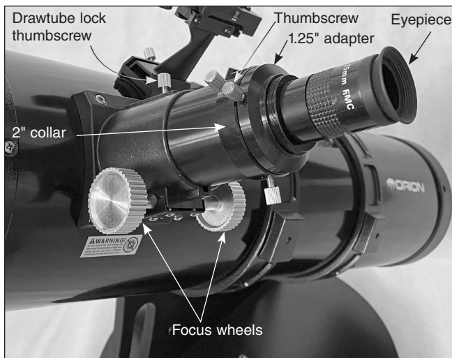
Figure 4. Insert an eyepiece into the focuser and secure it by lightly tightening the thumbscrew..
