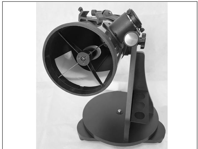
Figure 12. Before collimating your telescope, place a piece of white paper inside the optical tube opposite the focuser. Make sure the telescope tube is oriented parallel to the ground during the collimation process. [StarBlast 4.5 Astro Reflector pictured]
