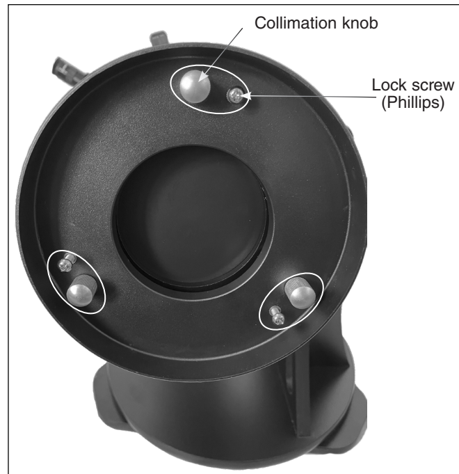
Figure 15. The optical tube's rear cell has three pairs of collimation screws for adjusting the tilt of the primary mirror. The large knobs are the spring-loaded collimation knobs while the smaller Phillips screws are the locking screws.
